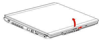
Figure 3-3 Opening the display panel
